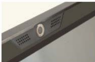
• Built-in 0.3 mega-pixel webcam with digital microphone (AFL-317A)
