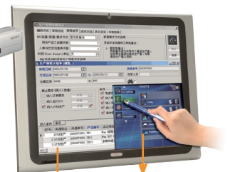
VGA Main Source-Production Management Software BNC Second Source-Surveillance Image
