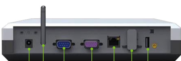
Serial Console (RS-232) Wireless LAN Antenna RS-232 VGA RJ-45 LAN SD CardSlot USB 2.0
