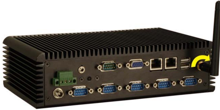
Figure 4-13: Wireless Antenna Installation
